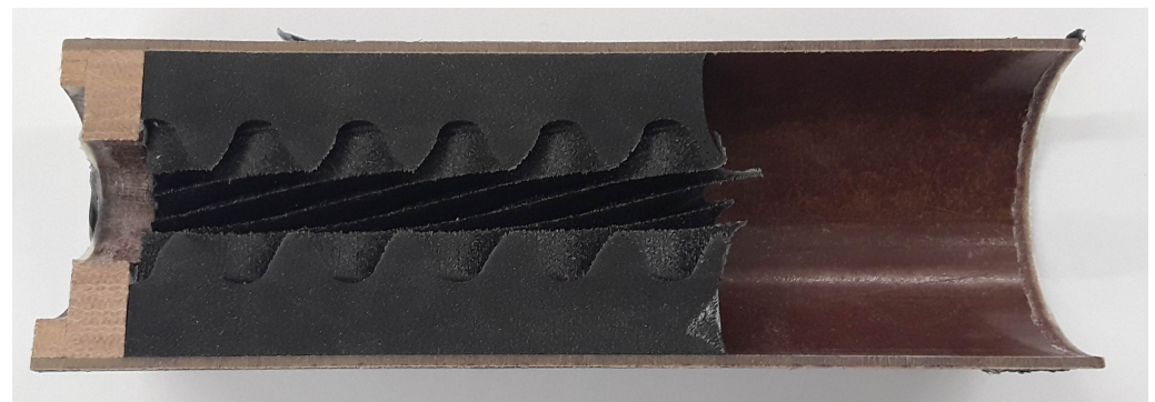
Figure 8. Sectional view of a test fuel block after the mold was dissolved.
