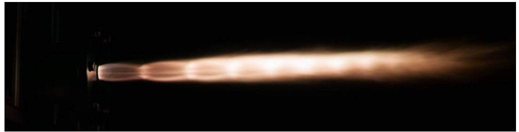
Figure 12. Side view of the jet blast with under expansion form a Monoport geometry.
