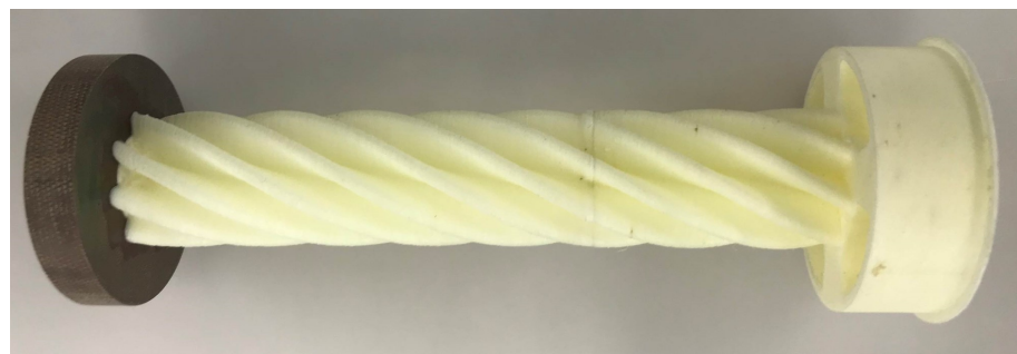
Figure 5. The two moldings are glued together (white-yellowish) and onto the vortex disk (dark brown) [16].
