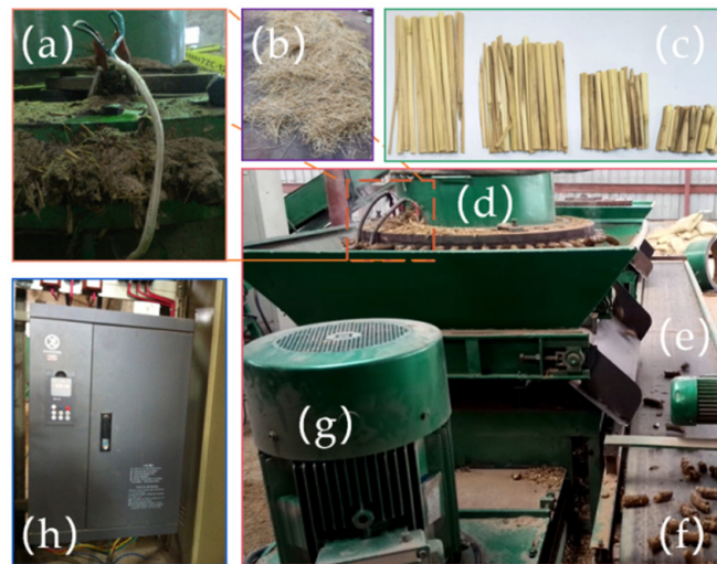
Figure 3. Schematic diagram of the briquetting process: (a) Electric heating tubes; (b) Dry straw; (c) Cut straw; (d) Briquetting machine; (e) Conveyor belt; (f) Briquette; (g) Motor; (h) Variable-frequency drive.
