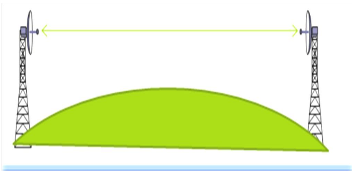
Fig. 1. Mobile communication propagation Line of Sight (LOS)
