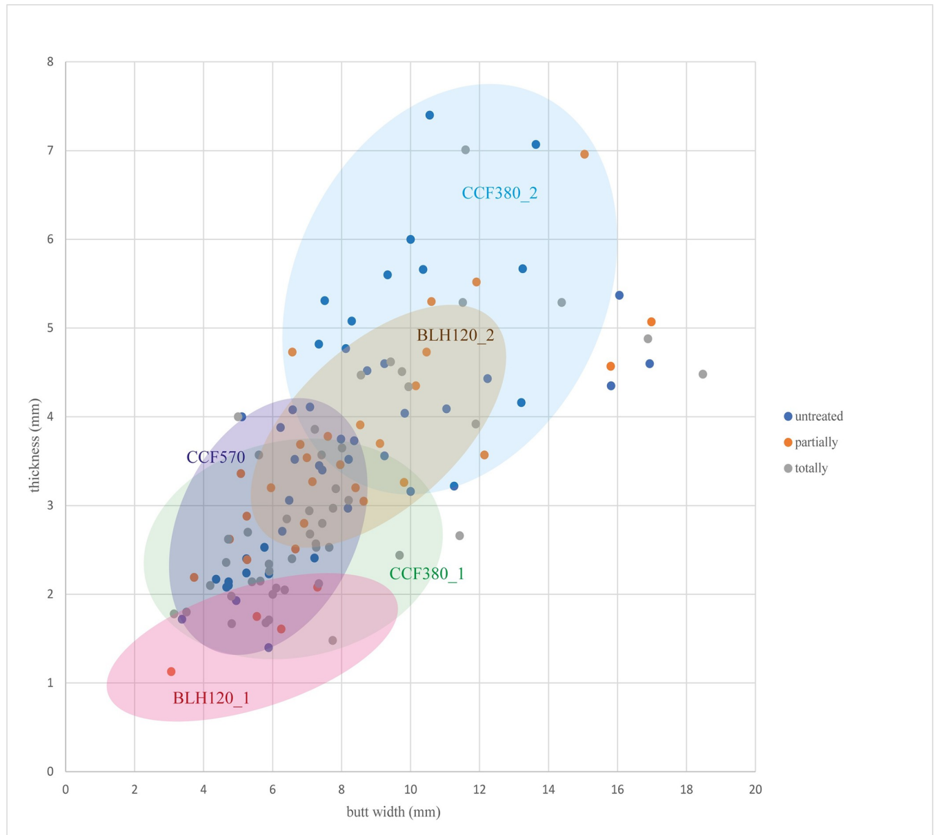
Fig 7. Comparison of ranges of the 5 recognized groups based on butt measurements by overhang preparation type.
