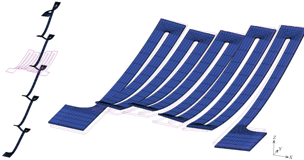
Figure 7. FE simulation of increment 8 in the experiment, where the boundary conditions in extended (left) and returned (right) state are derived from the measured topographies.
