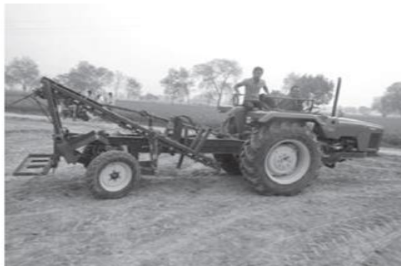
Fig. 3. Tractor mounted carrot digger developed by Naresh
